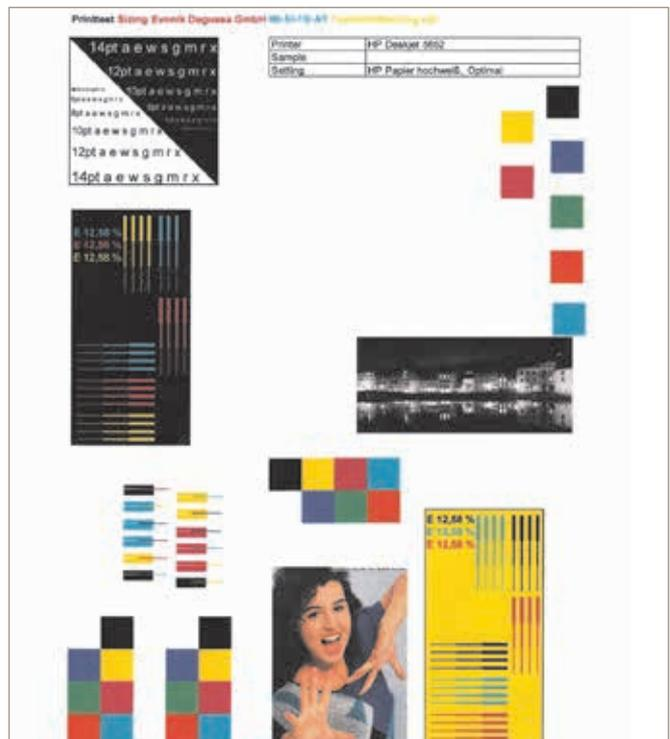
Color density and L\*a\*b\* values were measured using both the SpectroEye and the PIAS device. The gamut area is calculated based on CIELAB a\* and b\* values for the different colored measuring areas.
