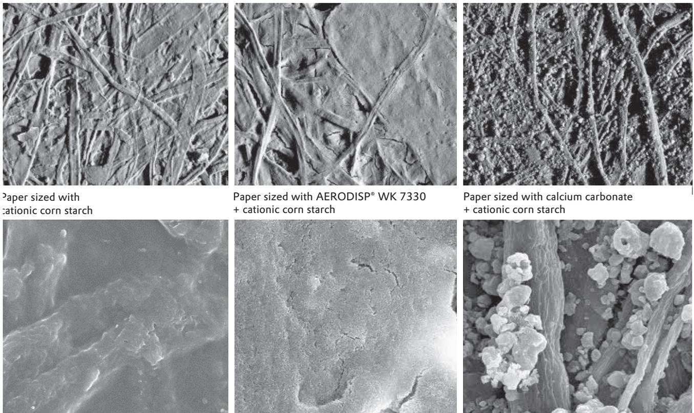
Nano-structured fumed silica creates a very thin yet smooth and porous coating that covers the paper fibers more or less completely. Dyes or color pigments are retained at the surface of the silica particles resulting in higher optical densities and an expanded color gamut area. As seen in the SEM micrographs, the paper surface is visibly more homogeneous, which in turn has a favorable effect on print resolution and ink uniformity.
