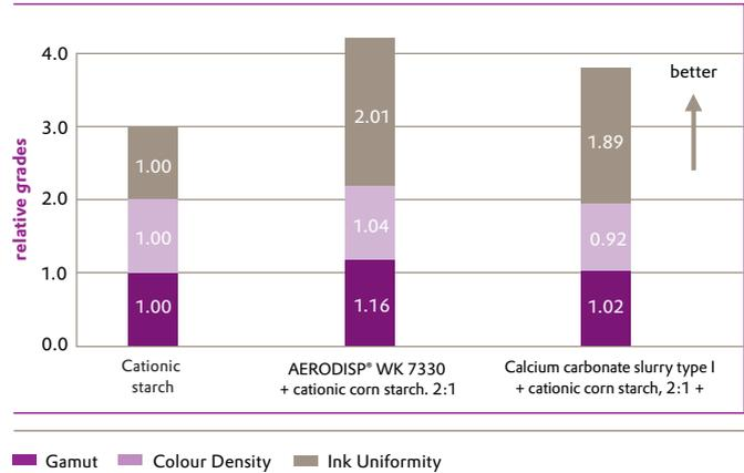
Different from colloidal silica, calcium carbonate can have a positive impact on print performance; however it is clearly inferior to AERODISP® in cationic sizing formulations (Figure 22).
