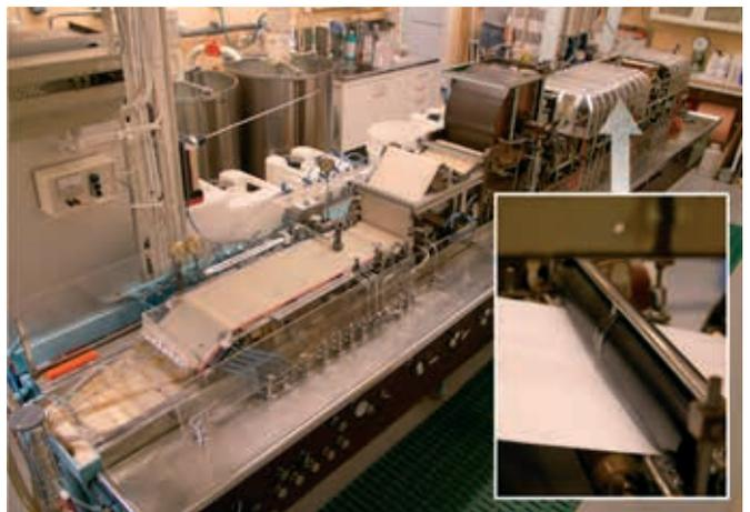
**Figure 8** Kämmerer paper machine "XPM" used for online-sizing trials. The small picture shows the puddle-type size press.
