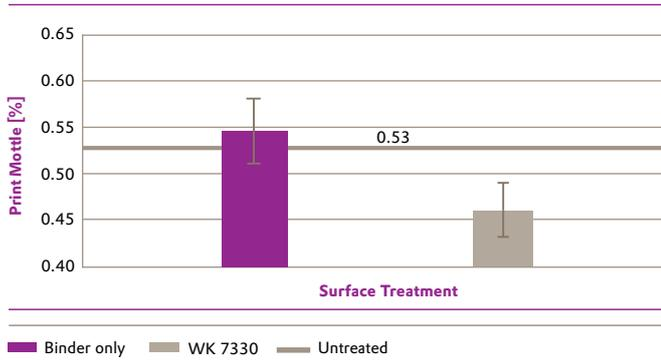
The results described in 4.7.1 and 4.7.2 demonstrate that paper sizing with AERODISP® not only improves the inkjet print performance but enables the manufacture of multi-functional papers which can be used on various printing platforms.
