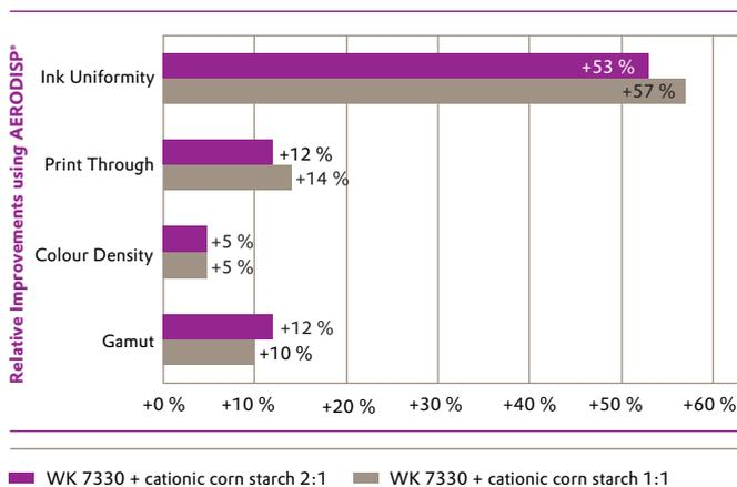
Similar results were found with non-ionic starch based formulations where AERODISP® had a positive impact on print performance and in particular ink uniformity (Figure 19).
