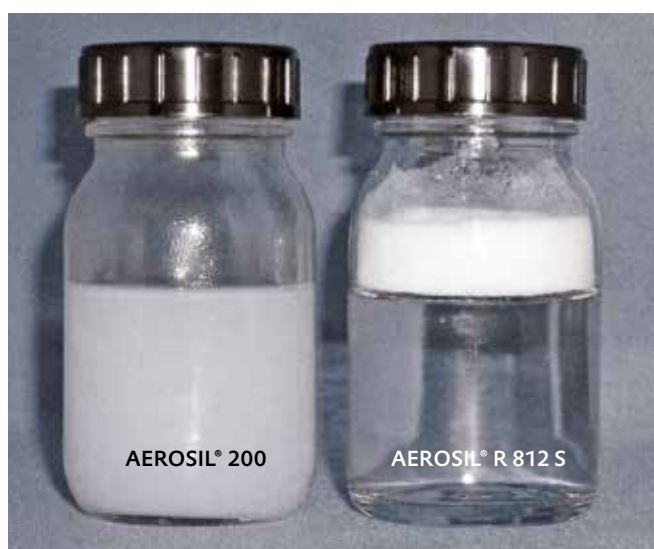
Figure 6 Behavior of AEROSIL® 200 (left) and AEROSIL® R 812 S (right) in the presence of water. AEROSIL® 200 may be readily dispersed in water, whereas AEROSIL® R 812 S is not wettable and floats on the surface of the water.
