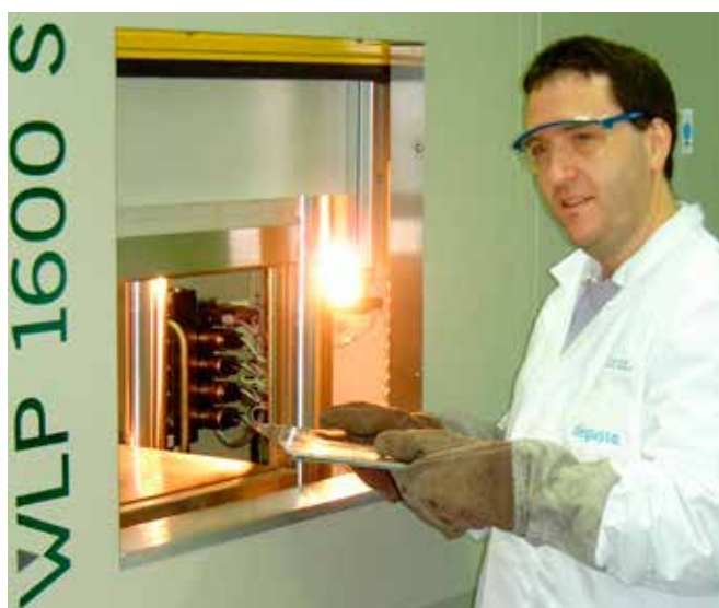
Figure 12 Vulcanization press; Manufacturer: Wickert Maschinenbau GmbH, Landau, Germany
