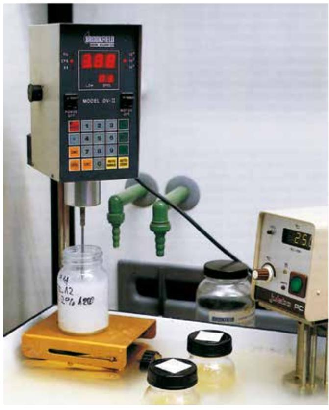
**Figure 9** Rotation viscometer DV-II of the Brookfield Engineering Laboratories, Inc., 240 Cushing St., Stoughton, MA 02072 USA
