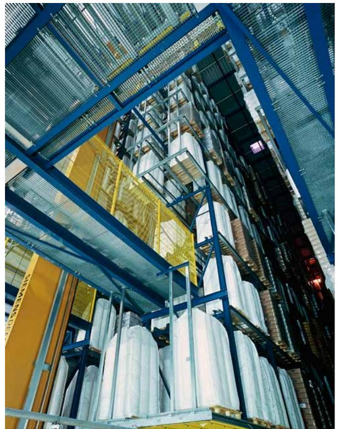
**Figure 9** Warehouse with high bay racking to store bags and FIBC
