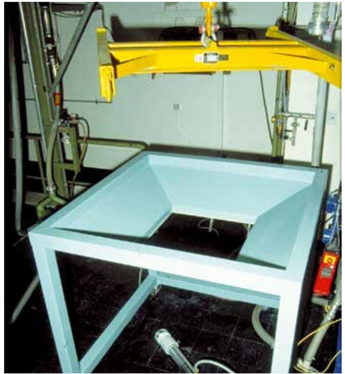
**Figure 8** Safety frame for FIBC discharge
