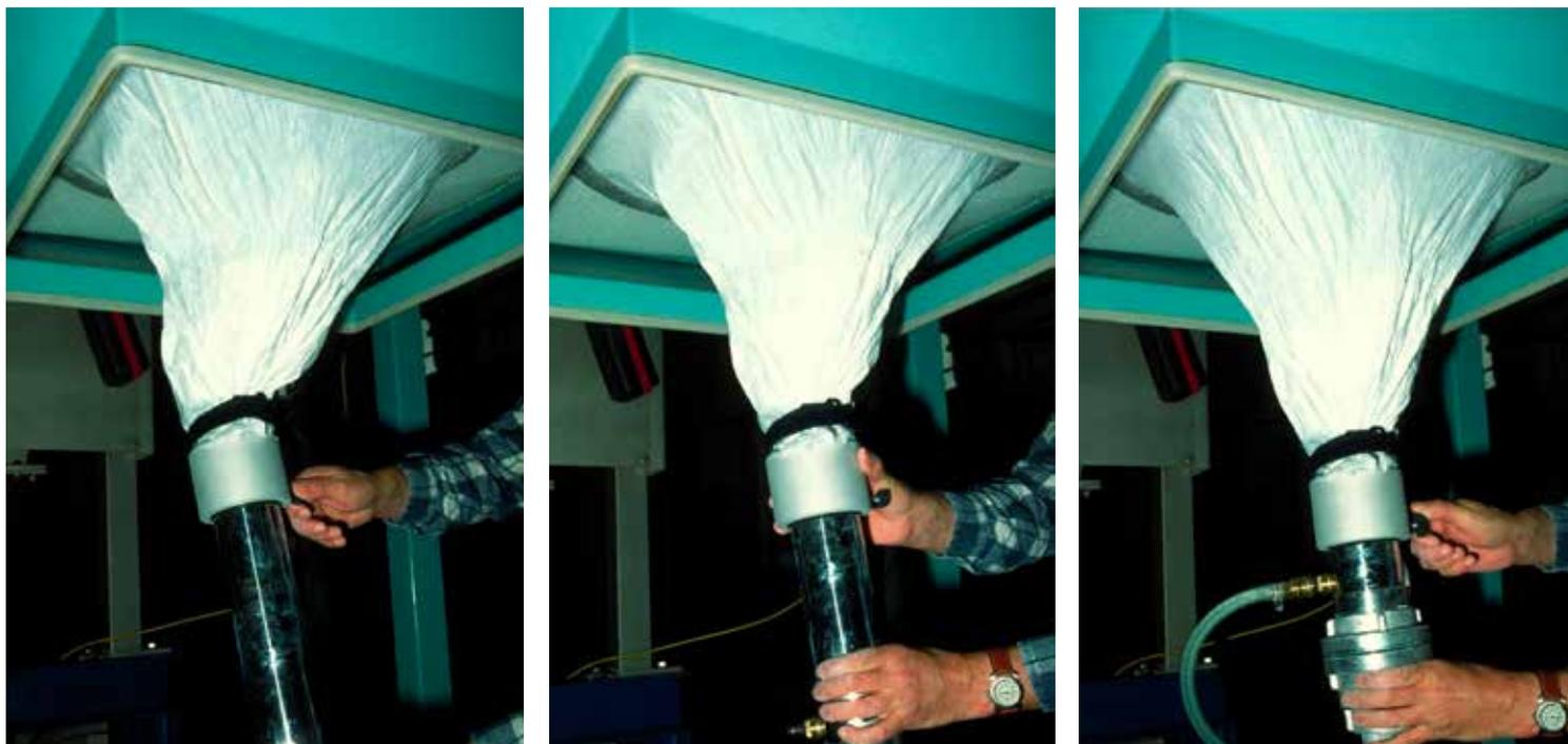
**Figure 15** Pushing the PESy into the FIBC
