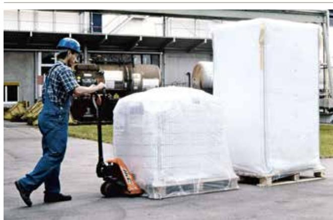
**Figure 3** 1 m<sup>3</sup> and 2 m<sup>3</sup> – FIBCs on CP3 pallet (114 cm x 114 cm)
