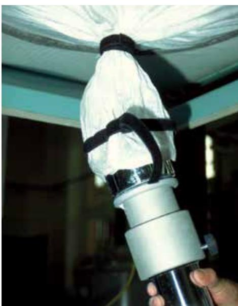
Now open the strap until the entire cross section of the outlet is released. Insert the PESy into the outlet as far as possible so that the mobile slide of the PESy moves into its frontmost position (see **Figure 12**).
