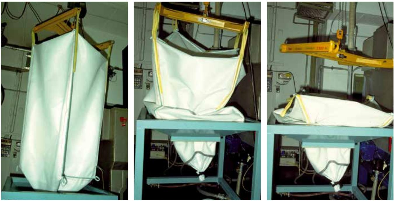
**Figure 24** Removing the FIBC from the lifting apparatus
