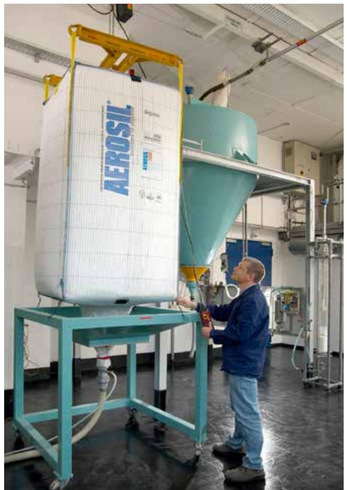
**Figure 9** FIBC before discharge
