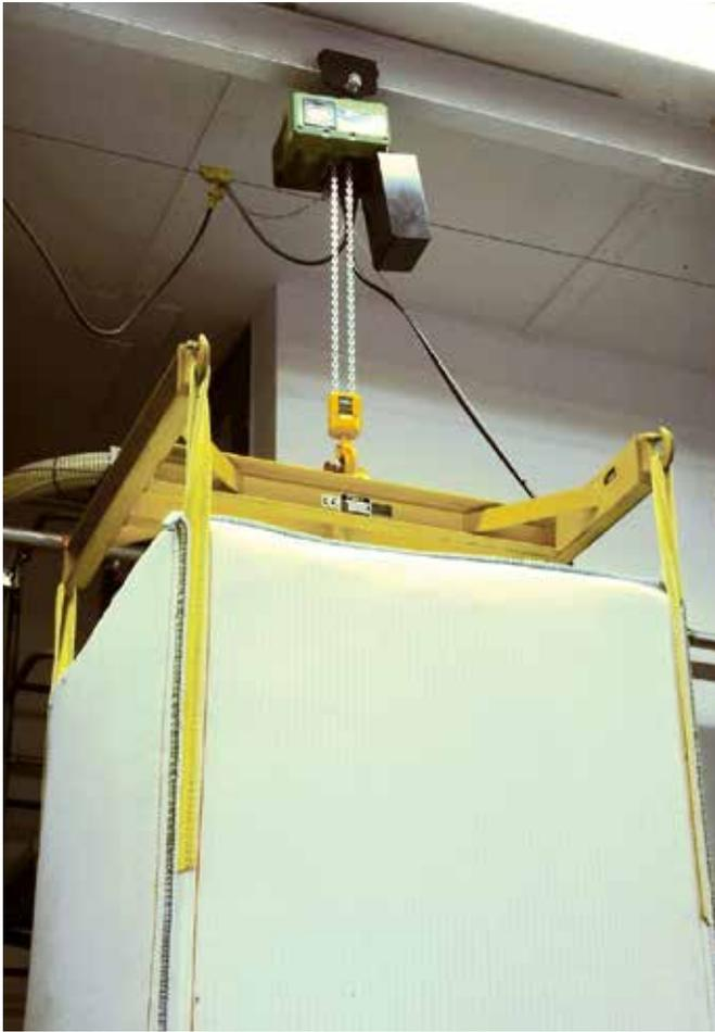
**Figure 7** Lifting yoke with safety hooks
