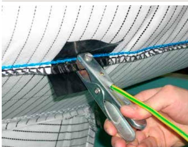
**Figure 10** Grounding the FIBC
