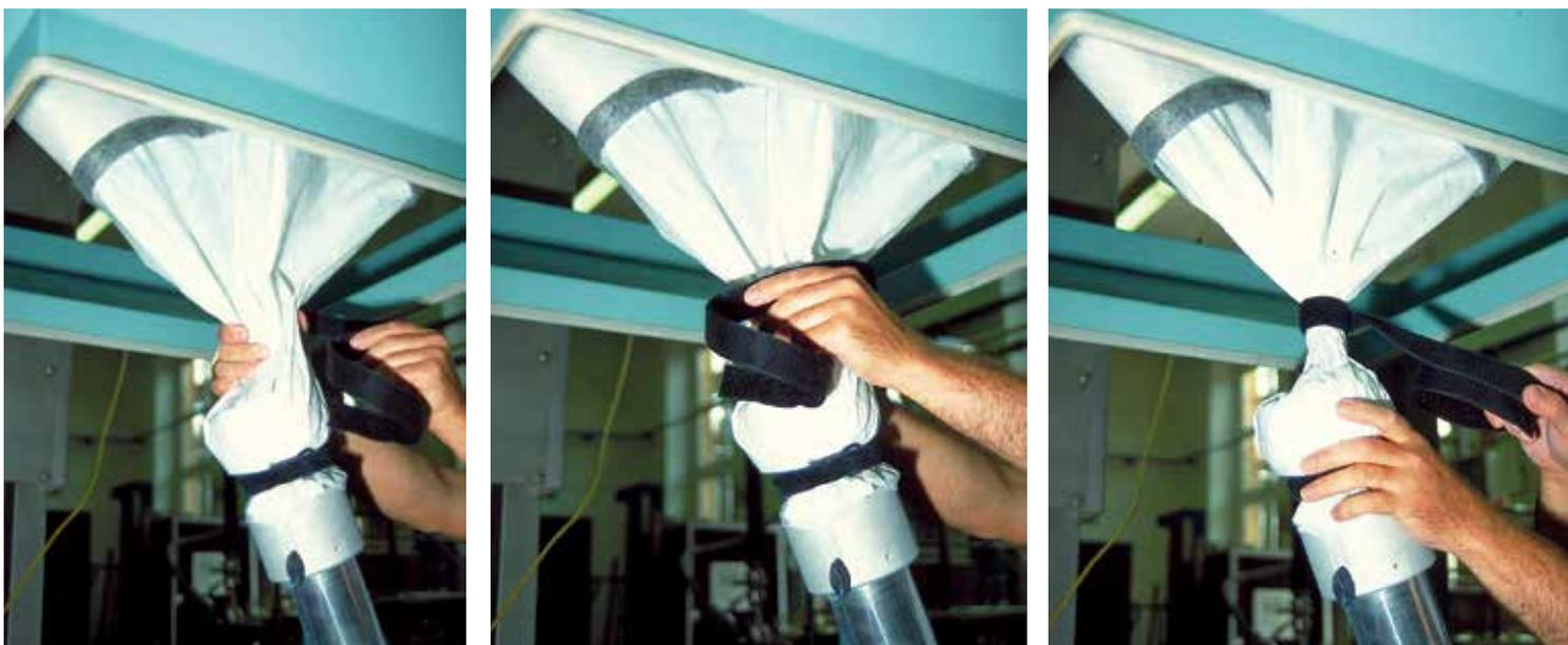
**Figure 21** Sealing the discharge spout
