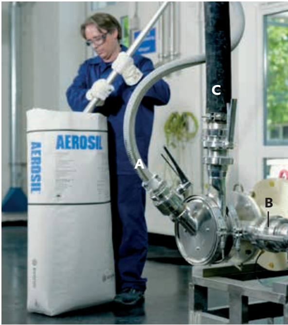
Figure 11: Continuous rotor-stator mixer showing the inlets for the AEROSIL® (A) and the liquid (B), and the outlet for the product (C). This system is practically dust-free.
