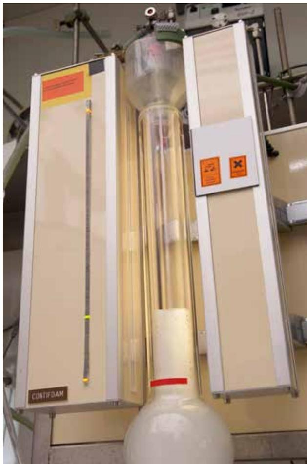
**Figure 9** Circulation test unit Contifoam (capacity of the glass vessel: 600 ml)
