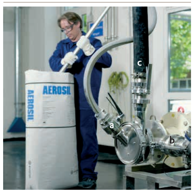
Figure 3.5 Continuous rotor-stator mixer showing the inlet for the AEROSIL® (a) and the liquid (b), and the outlet for the product (c). This system is practically dust-free
