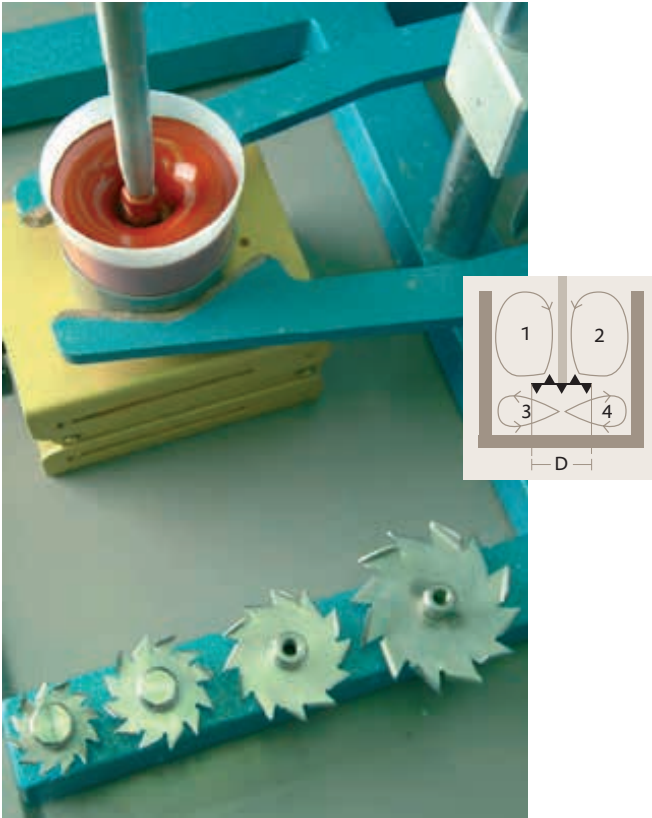
Figure 3.1 Dissolver (chopper or toothed disk). For best results, the container should have a diameter at least twice that of the disk, yet not be too large. The dispersion shown on the picture was colored for better visibility.
