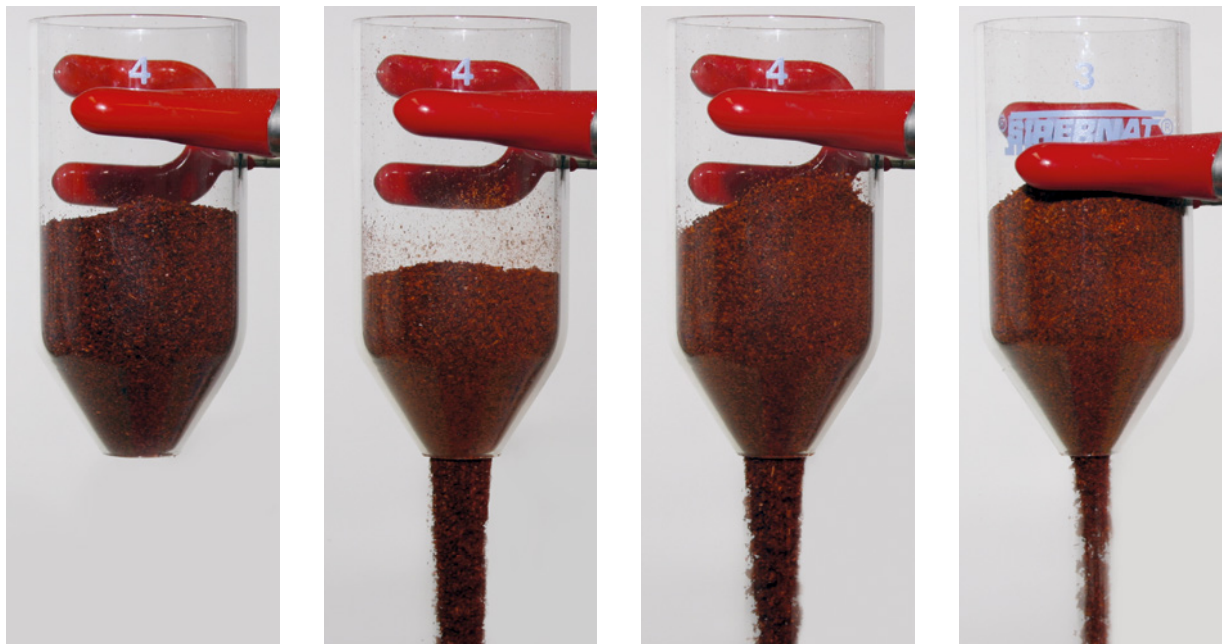
Picture 1 Measuring the flow grade of various Chili powders. From left: Untreated raw material; treated with SIPERNAT® 350; treated with AEROSIL® 200F; treated with SIPERNAT® 50S
