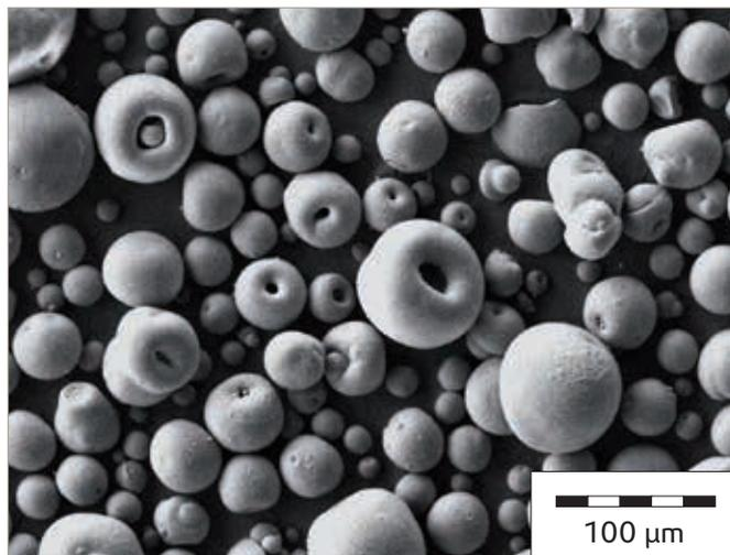
**Figure 2** Scanning electron microscopy image of AEROPERL® 300 Pharma
