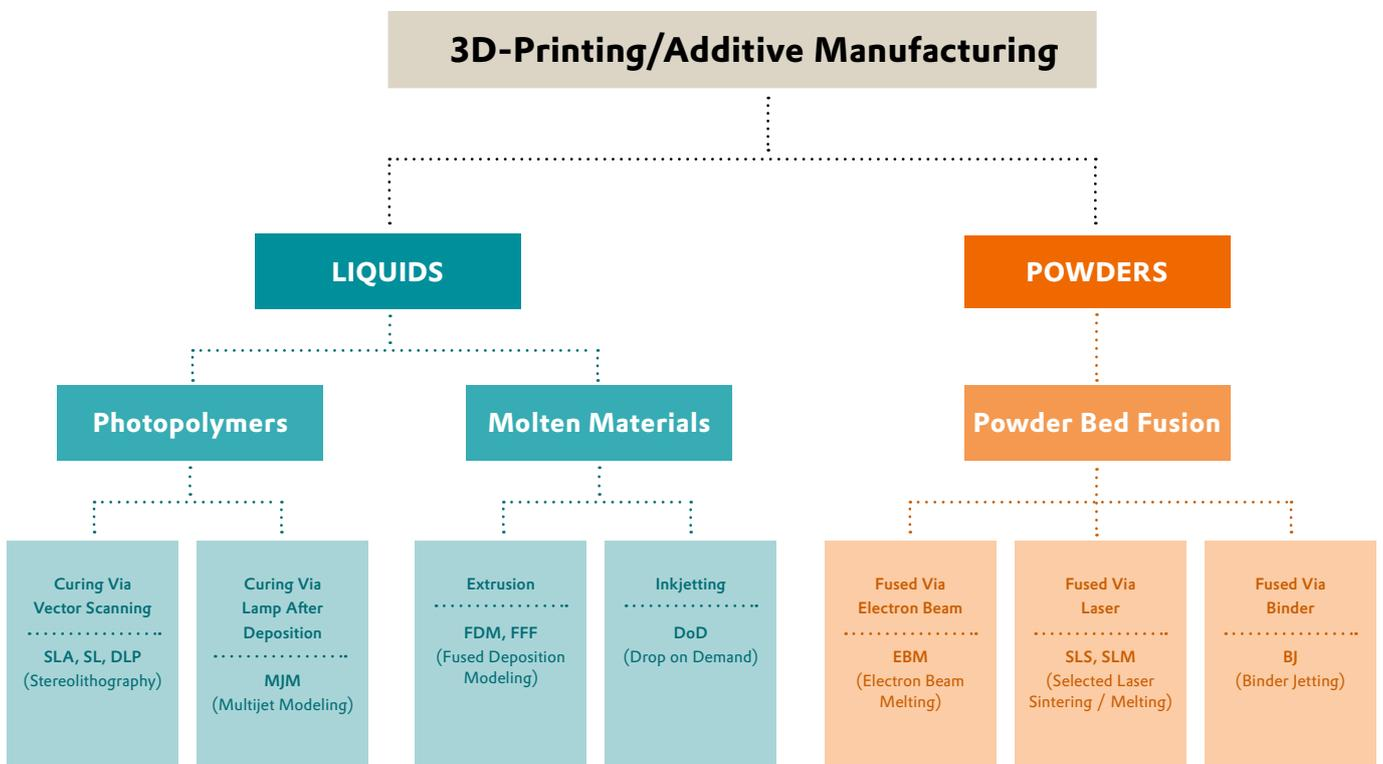
**Figure 1:** Brief classification of technologies often used in 3D printing / additive manufacturing. Abbreviations of the specific technologies do not cover all terms used. Abbreviations and technical terms are often based upon technical terms registered under <sup>TM</sup> or ©. 1
