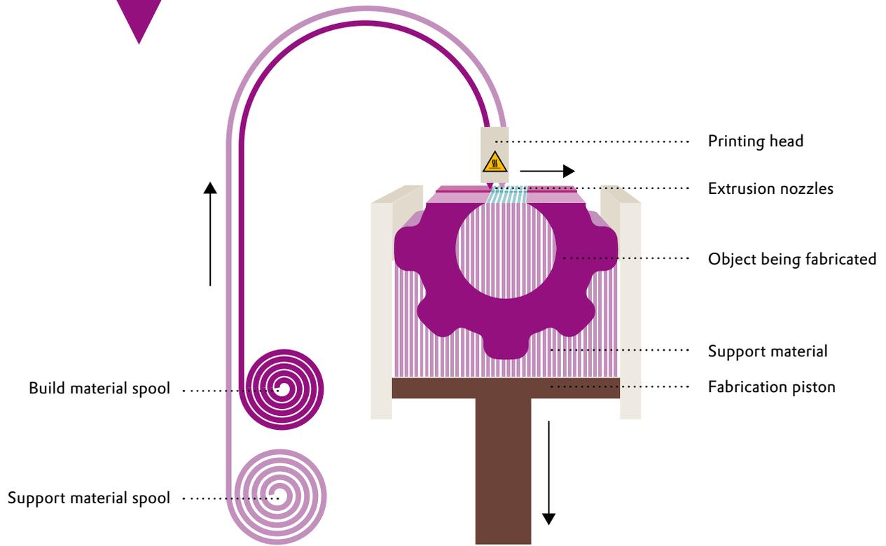
**Figure 10** The basic principle of material extrusion using building material and support material
