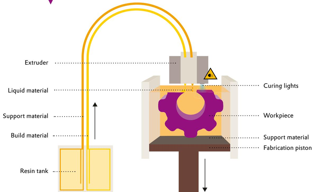
Figure 4 Schematic drawing of a Polyjet process
