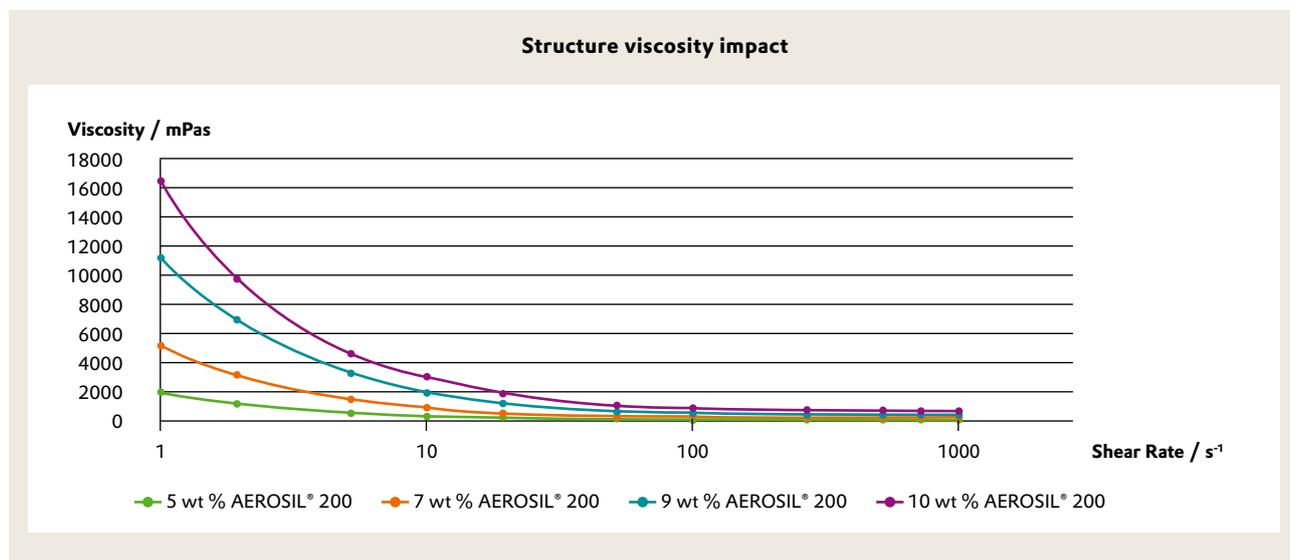
Figure 13 Structure viscosity impact of AEROSIL® 200 addition in unipolar media.
