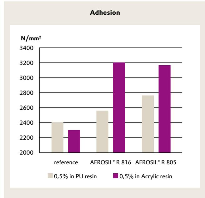
**Figure 11** Surface treated AEROSIL® grades help to increase adhesion of the layered structures and thus prevents from delamination of the final structure.
