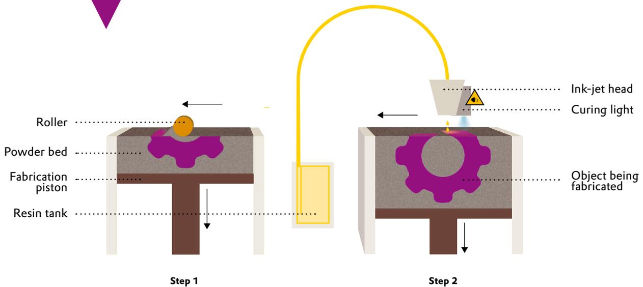
Figure 12 The two-step process in binder jetting.
