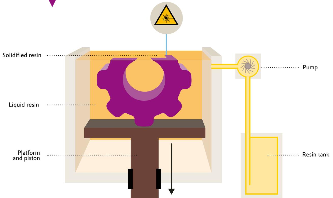
Figure 2: Schematic drawing of the vat polymerization process.
