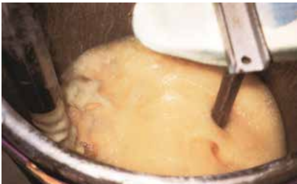
Picture 8 Mixing of 7% AEROSIL® 200 in Palatal M 671-01V (tamped density of 50 g/l)
