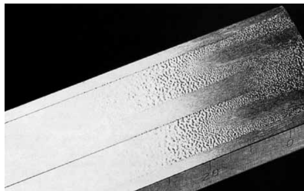
Picture 4 AEROSIL® polyester resin dispersion with a grind reading of approx. 40 µm
