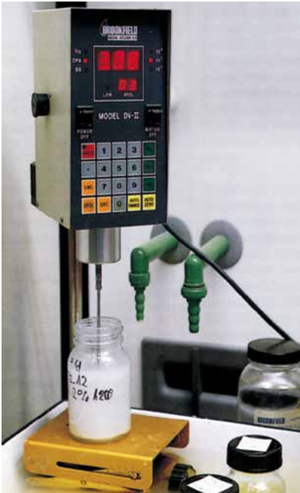
Picture 2 Rotational viscosimeter DV-II (Brookfield Engineering Laboratories, Inc., Stoughton, MA, USA, German representative: Brookfield Engineering Lab. GmbH, D-73547 Lorch)
