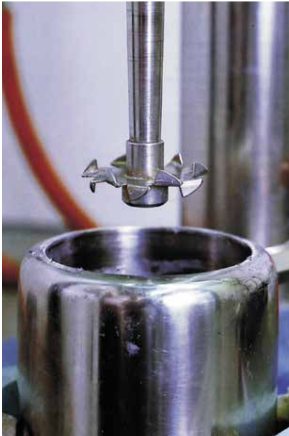
Picture 5 Lab dissolver blade (Cowles Division, Morehouse, New York, USA)
