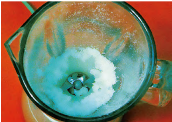
Figure 7: Choline chloride paste created by shearing of the formula shown in figure 8
