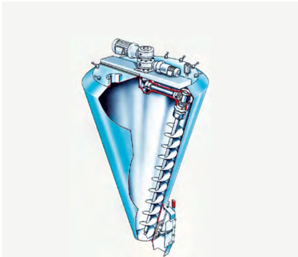
Figure 3: Schematic illustration of a Nauta® Mixer Hosokawa Micra B.V. Gildenstraat 26, NL-7000 AB-Doetichem, The Netherlands
