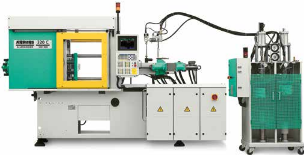
Figure 3 LSR injection molding machine; Manufacturer: ARBURG GmbH + Co., Lossburg, Germany
