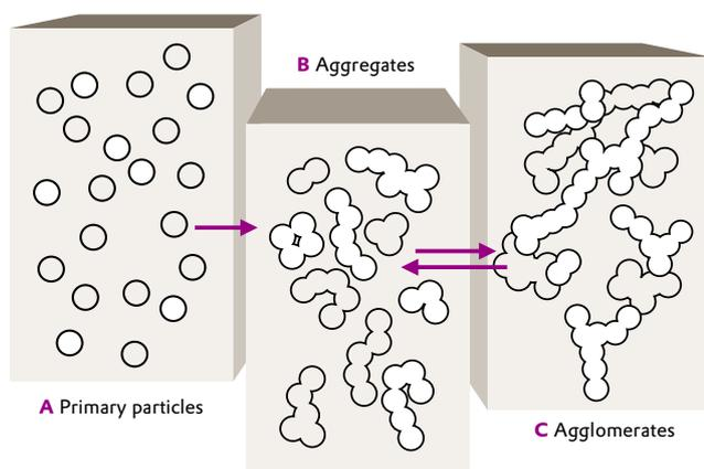
The aggregates are the smallest actual units of colloidal silicon dioxide. Once the aggregates cool down to below the fusion point, additional collisions result in mechanical entanglement and bonding of the chains, called agglomeration. Because agglomerates (Figure 1c) are only bound through weak forces, they can easily be broken down to aggregates during mixing or dispersion.
