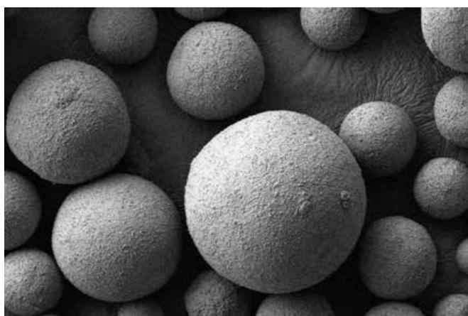
**Figure 4** Scanning electron microscopy image of AEROPERL® 300 Pharma
