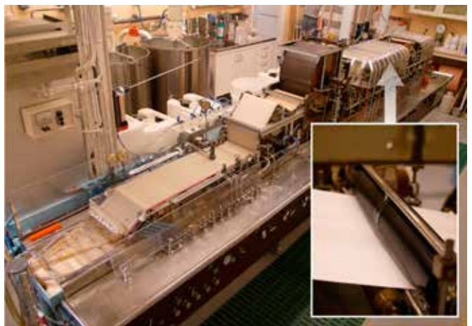
Figure 8 Kämmerer paper machine "XPM" used for online-sizing trials. The small picture shows the puddle-type size press.
