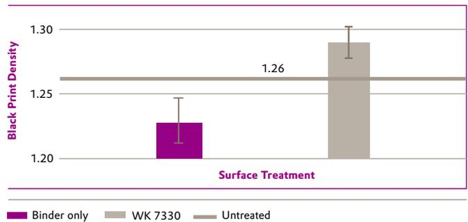
**Figure 26** Print uniformity, on a fine scale improves when AERODISP® is added to the sizing agent(s), as seen by the reduction in print grain
