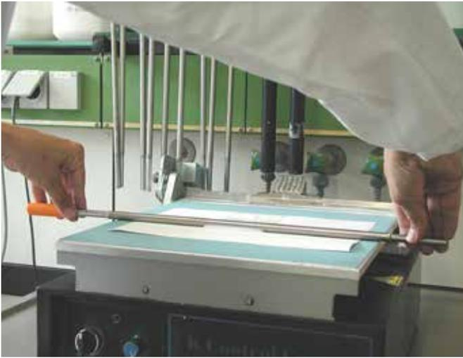
**Figure 6.1** Manual paper coating in the laboratory
