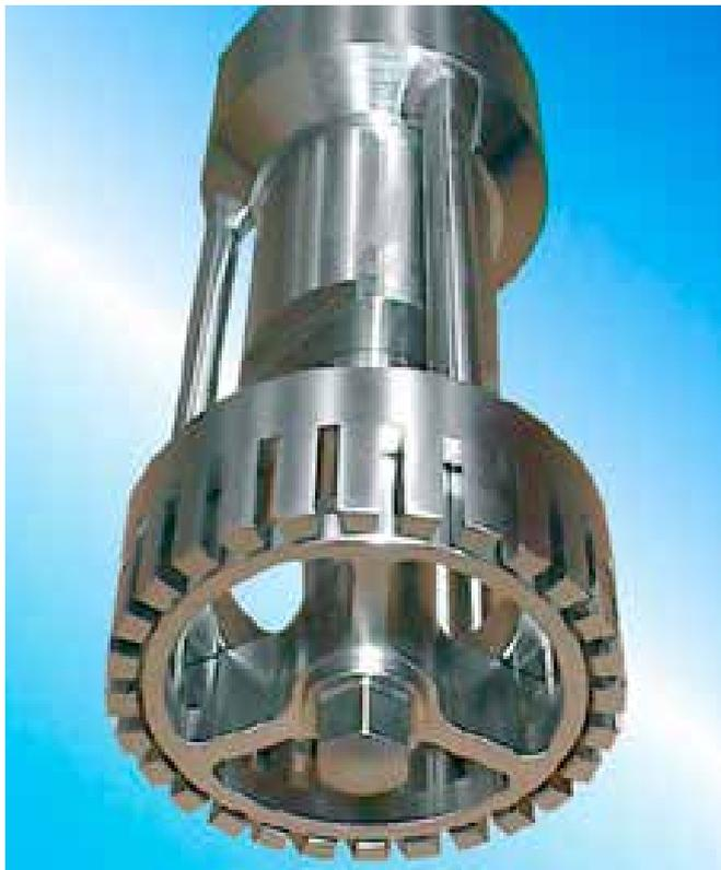
**Figure 3.4** Rotor-stator mixing head
