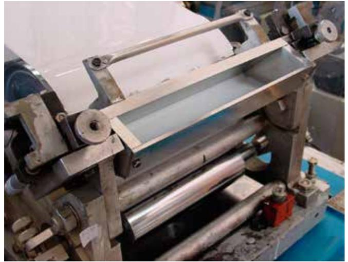
**Figure 6.2** Paper coating with a casting knife
