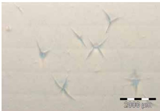
**Figure 8.1** Microcracking
