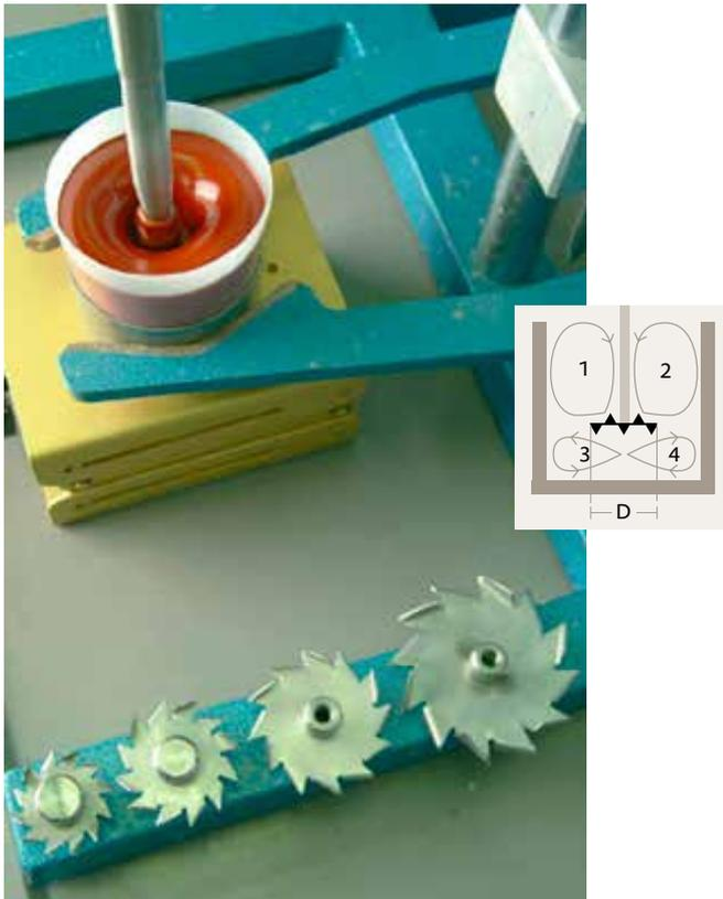
**Figure 3.1** Dissolver (chopper or toothed disk). For best results, the container should have a diameter at least twice that of the disk, yet not be too large. The dispersion shown on the picture was colored for better visibility.
