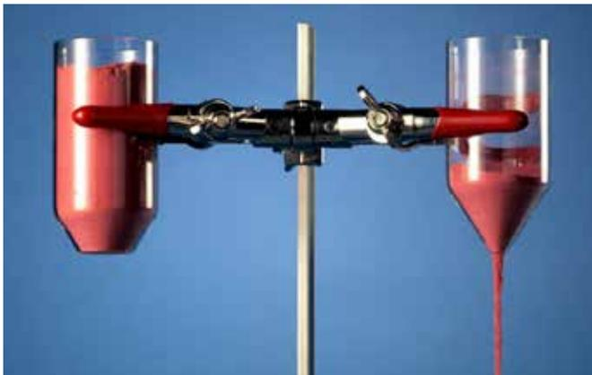
**Figure 5** Flow funnels to determine flow grades
