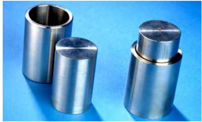
**Figure 6** Steel cylinder to determine caking tendency
