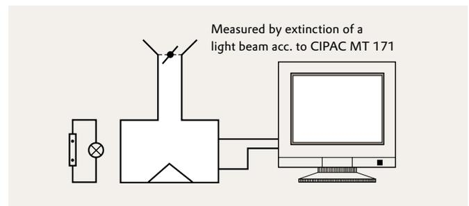
**Figure 7** Model of dust measurement by optical method
