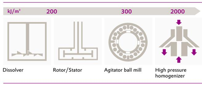
The dispersing time and the rotational speed of the dispersing equipment should be adjusted as well as the type of AEROSIL®. Some types such as AEROSIL® 380 are more resistant against high shear forces than AEROSIL® 200. Higher surface area AEROSIL® grades such as AEROSIL® 300, 380, and AEROSIL® R 812 S require more energy-intensive mixing equipment for optimized dispersion. For most applications peripheral velocity can be more than 7 m/sec using a dissolver or a rotor stator system.
