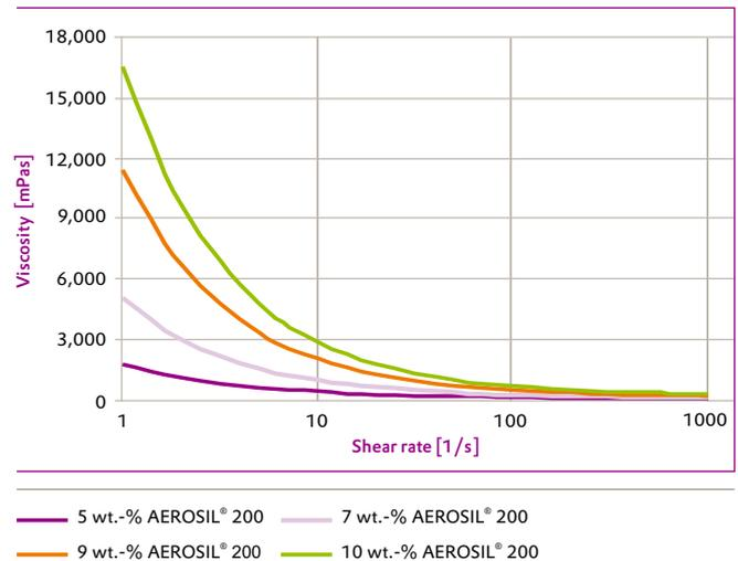
**Figure 5** shows the thickening performance achieved using the basic type AEROSIL® 200 in paraffin oil. The higher viscosity level in the non-polar oil is reached with lower AEROSIL® 200 concentrations compared to the viscosity level in the more polar soybean oil.
