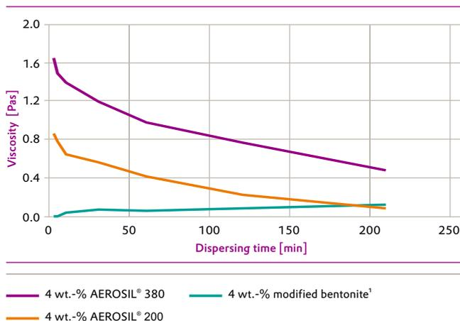
The figure shows clearly the advantage of shorter dispersing time when AEROSIL® fumed silica is used. This reduces production time and therewith manufacturing costs. Air bubbles incorporated during the dispersion process should be removed by generating a vacuum. If a higher viscosity level is needed, this can be obtained through increasing the concentration of AEROSIL® fumed silica.
