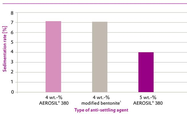
The sedimentation rate was measured by a slide gauge and calculated in percent relating to the height of sample bottles Schott Duran 50 ml (SCHOTT AG/Germany) minus the height of the bottom (30 mm) of the sample bottles.
