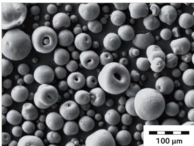
**Figure 2** Scanning electron microscopy image of AEROPERL® 300 Pharma
